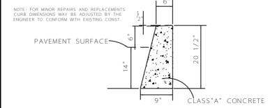
TYPICAL CROSS - SECTION OF CURB WITHOUT GUTTER
